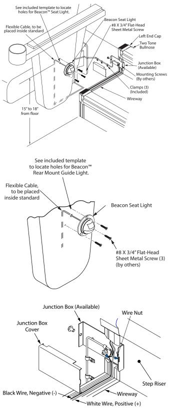
Junction Box Wiring Detail
